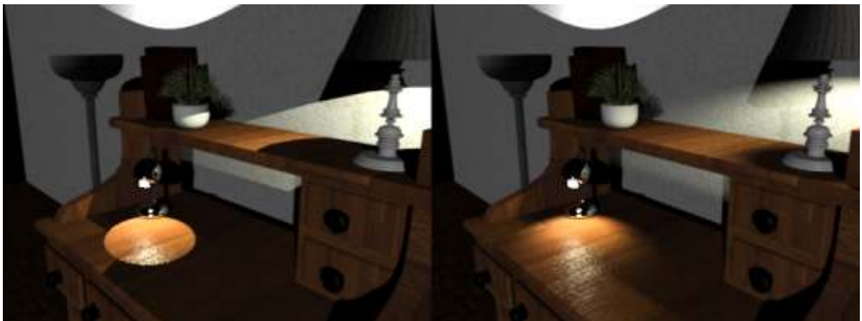
Fig. 5.2 - Simple scene rendered with area lights approximated by point lights (left) and full area light sampling (right)
