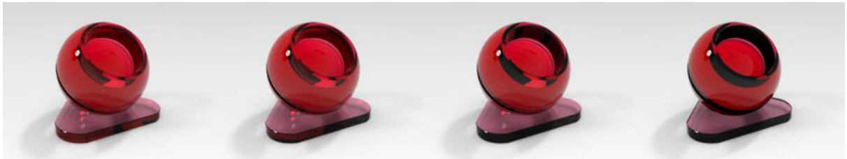
Fig. 5.4 - From left to right: A glass object rendered with different trace depths 8, 6, 4 and 2
